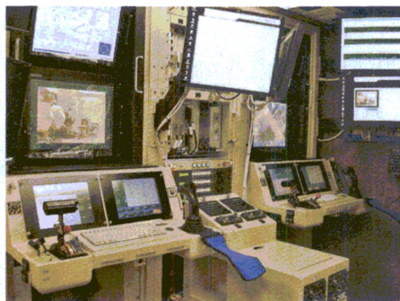
4. For the latest in UAS-guided control, advanced cockpit controls must be deployable to be within reach of the UAS's communications link. (Courtesy of General Atomics Aeronautical)
